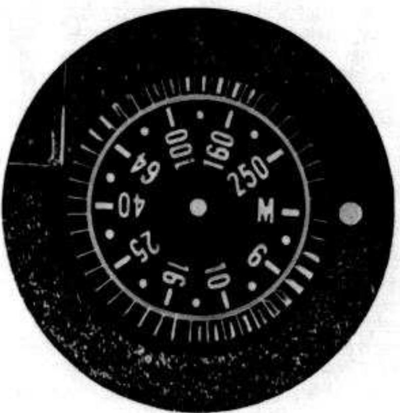
Set the film speed dial to 'M'. Then, by moving the manual exposure lever toward manual, you can set the lens opening you choose (2·3, 2·8, 4, 5·6, 8, 11, 16). The red needle in the exposure indicator determines the exposure you choose. By setting your lens manually, you can get special exposure effects as described on page 27.
