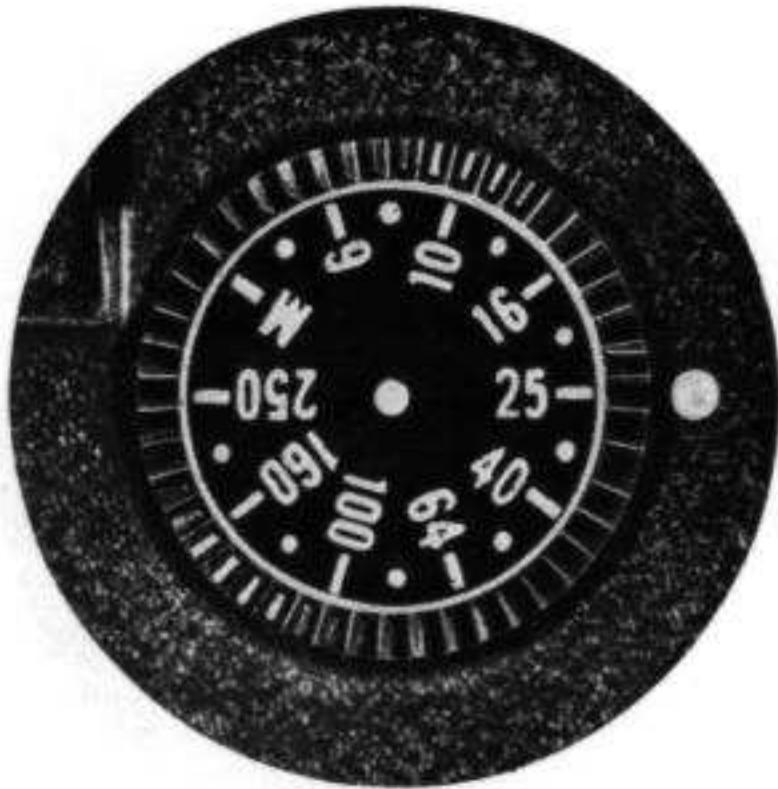
Your camera has a graduated scale with film speed settings from 3 to 250. To set the Optronic Eye for the correct film speed, turn the dial until the correct film speed is opposite the indented dot (Arrow). You will find the recommended film speed on the instruction sheet packed with the film. The indoor film speed rating is usually different than the outdoor rating on most films. Be sure to set the Optronic Eye at the correct speed. Manual Operation (M) is explained on page 20.
