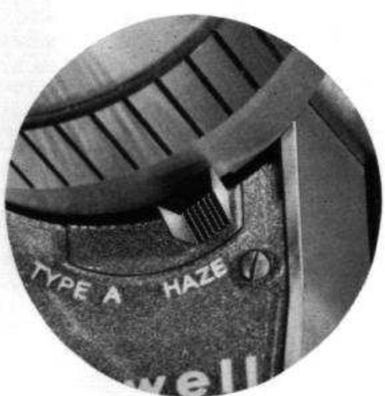
Your camera provides both 'Haze' and 'Type-A' filtering. Set the Filter Lever to the 'Haze' position which you'll use most of the time, whether you're filming indoors or out.
