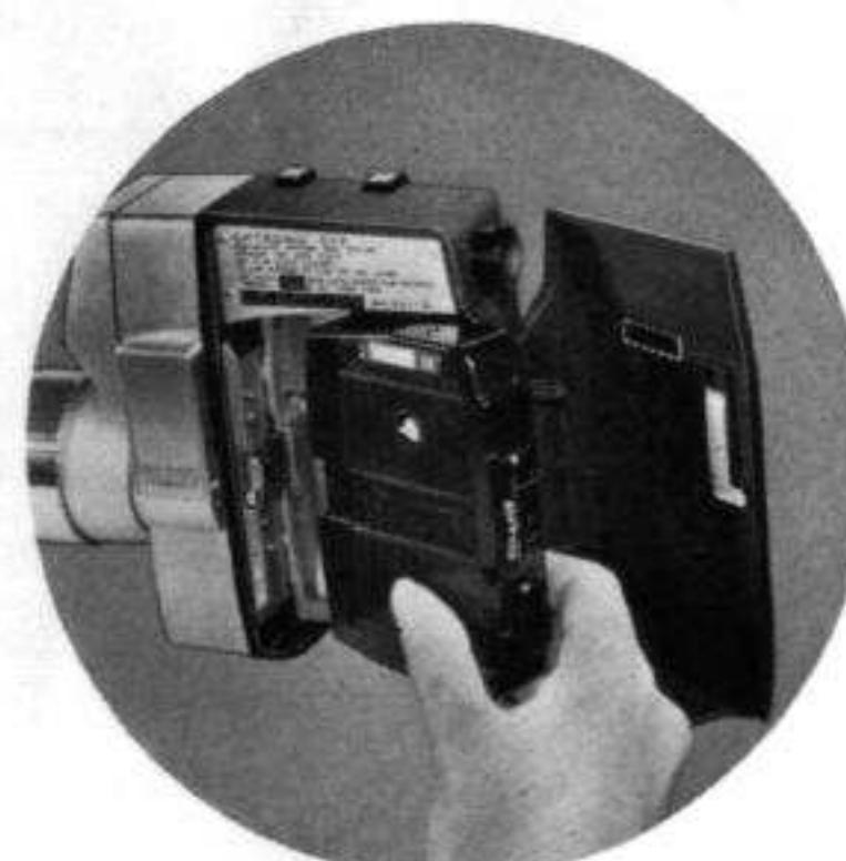
After you have exposed the first 25 feet of film as shown on the Footage Counter, wind the camera, and run until it stops. The automatic stop in the cartridge will stop the camera with the Footage Counter at 'End'. Open the camera door and remove the cartridge. Absolutely, do not open the cartridge. Note that '1' appears in the Side Exposed Window.
