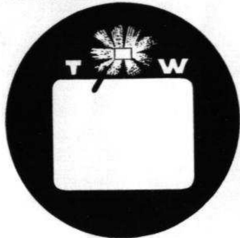
Look through the viewfinder. The Exposure Beacon (top centre) when red, indicates insufficient light for proper exposure. If yellow, there is enough light for correct exposure. Do not use the Exposure Beacon as a guide when the ASA dial is set to (M), or when the manual control lever is not on 'automatic'.
