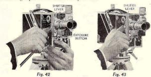
MAKING A "FADE-IN:" Set the SHUTTER LEVER at CLOSED. Push in the exposure button in the usual way. The instant the motor starts, slowly move the SHUTTER LEVER to OPEN, as shown in Figure 42. While the lever is being moved, the "fade-in" occurs. Therefore, the speed of the "fade-in" depends upon the speed at which the shutter is opened.
