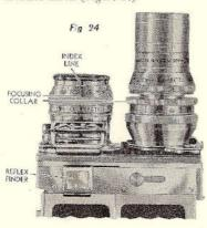
Another method of focusing the Ciné-Kodak Special is to use the REFLEX FIND-ER and to focus visually. This obviates estimating distances. Use of the reflex finder is described on page 42. DEPTH OF FOCUS: When the lens is focused on a given distance, objects somewhat
