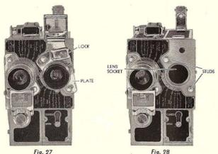
HOW TO REMOVE AND ATTACH LENSES: Remove the protective cap and plug before attaching lenses. To remove a lens from the turret, push the LOCK up and to the left, so that the PLATE will be at an angle, as shown in Figure 27.
