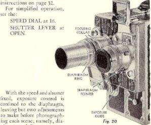
With the speed and shutter fixed, exposure control is confined to the diaphragm. leaving but two adjustments to make before photographing each scene; namely, diaphragm and distance:
