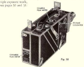
CHAMBER FILM METER. This meter operates on the circumference of the supply roll of film and requires no setting. Its purpose is to indicate the amount of unexposed film in the chamber, whether the latter is on or off the camera.
